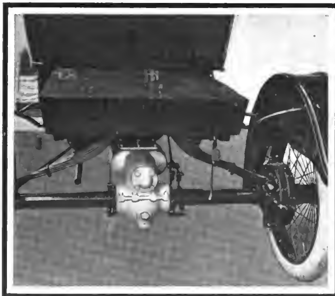
Rear axle and spring of B. S. A. car
